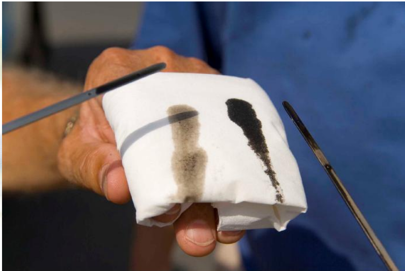
GTL burning Raider's oil on the left after 11000 odd km and a cruiser's oil on the right after only 4500 km - Doha - Qatar - 4-6-2006
